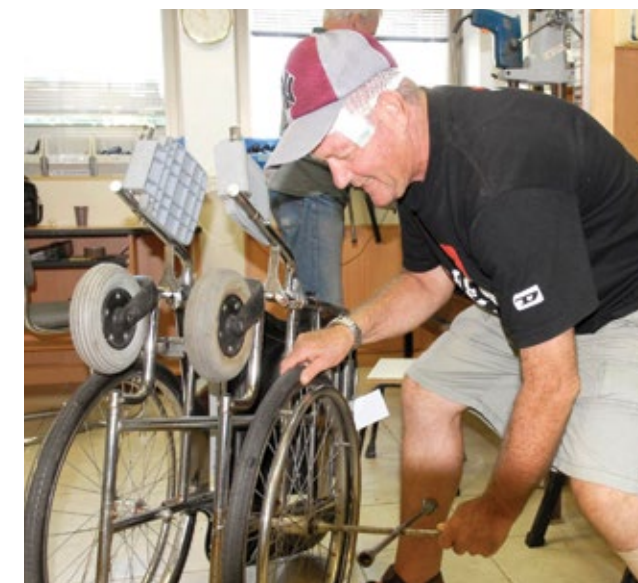
Some wheelchair repairs are simple – like tightening the bolts that keep wheels aligned.
